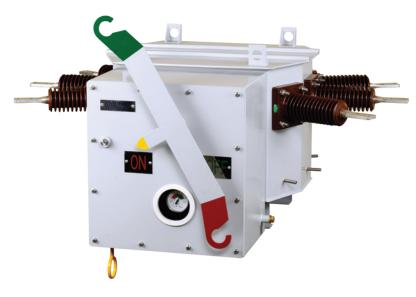
Pole Mounted Sectionalizer is dedicated to serve the purpose of disconnecting the faulty section automatically in conjunction with an upstream Autorecloser circuit breaker in the substation and restoring power to the healthy lines/branches with minimum down time.
