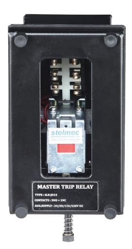
The Stelmec make SLR JH13 is an Electromechanical High Speed Tripping Relay used in tripping and signaling circuits of protective relays, where a high degree of reliability & high contact rating is required. It is an instantaneous switching element that is used for contact multiplication of Protection Relays of Circuit Breakers, thereby providing number of simultaneous instantaneous switching operations.
