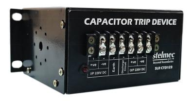
The Stelmec make SLR CTD123 is a Capacitor Trip Device used to trip the medium voltage 33/11Kv circuit breakers as DC supply fails by using the stored energy in a capacitor.
