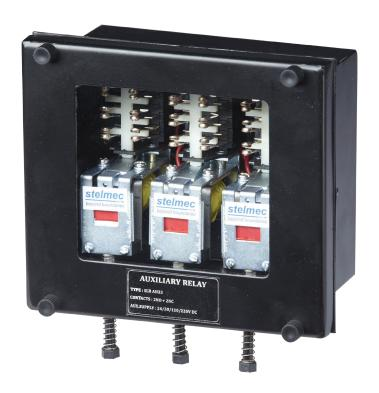
The Stelmec make SLR AH33 is an Electromechanical Three Element Voltage Operated (24/30/110/220)V DC Auxiliary Relay with 2NO and 2NC hand reset contacts and flag for Transformer Protection such as Buchholz relay trip / alarm, Winding Temperature trip / Alarm, Oil Temperature trip / Alarm etc.
